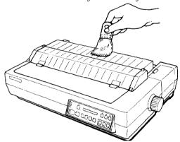
4. If the outer case or printer cover is dirty or dusty, clean it with a soft, clean cloth dampened with mild detergent dissolved in water. Keep the printer cover in place to prevent water from getting inside the printer.
